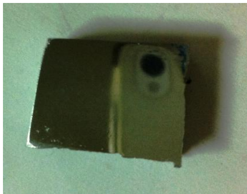
Fig. 4. Specimen for metallurgical test as crystal clear shown the mirror image of camera
