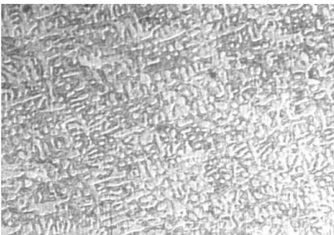
Fig. 11(b). Micrograph of Aluminum alloy sand cast at pouring temperature of 900 °C with high permeability of sand (x15)
